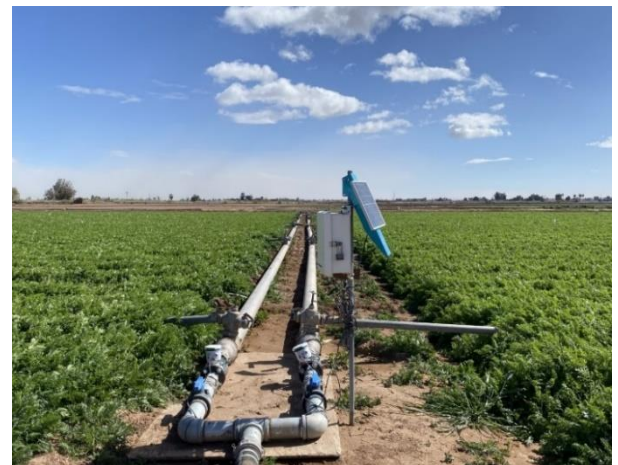
Fig. 3. Magnetic flowmeters and data store and transfer equipment to monitor water applied to the 22-23 trial.
