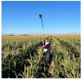
**Fig. 2.** A UCCE research staff is taking canopy infrared images to develop canopy growth curve for the desert sweet corn production systems.
