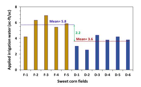
**Fig. 4.** Seasonal applied irrigation water in the furrow irrigated trial fields (F-1 to F-5) and the drip irrigated trial fields (D-1 to D-6). The mean values of seasonal applied irrigation water in each group of furrow and drip irrigated fields are also demonstrated.
