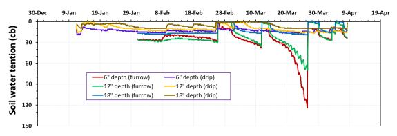
**Fig. 5.** Soil water tension at one drip irrigated sweet corn field against one furrow irrigated sweet corn field over the 2021-2022 season. The data is reported for the depths of 6, 12, and 18 inches for both fields. Maintaining soil water tension at a range of 20-30 centibars (cb) during mid-January through early-April is recommended for most experimental sites.
