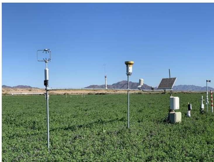
Figure 1. A fully automated ET monitoring tower at field 4. A total of 30 various sensors were installed above the canopy and at multiple depths of the crop root zoon at each site.
