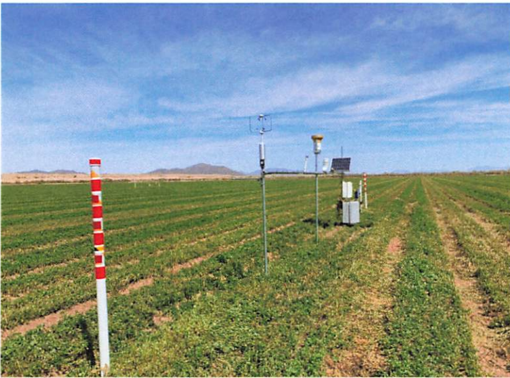
Figure 2. Fully automated surface renewal and eddy covariance ET station at the experimental field in the Palo Verde Valley.
